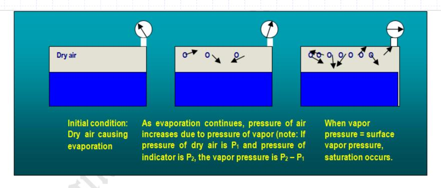
Denoting e as the vapor pressure and  $\mathbf{e}_{\mathrm{s}}$  as the saturated vapor pressure, the relative humidity is defined as,
