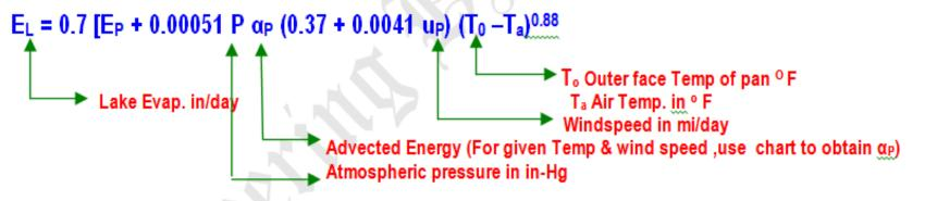
$$\underline{\alpha_P} = 0.13 + 0.0065T_0 - (6.0 \times 10^{-8} T_0^3) + 0.016 u_P^{0.36}$$
