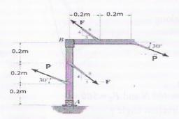
10. Determine the required magnitude of force **F** if the resultant couple moment on the frame is 200 N.m. clockwise and **P** = 1630 N.
