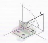
4. The force F acts on the bracket as shown. If the magnitude of the x and z components of F are  $F_x = 400 N$  and  $F_z = 500$ N, respectively, and  $\beta = 60^{\circ}$  find the coordinate direction angle  $\gamma$ .
