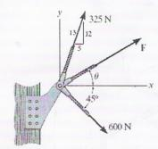
2. If the resultant force acting on the bracket is to be 800 Ndirected along the positive x-axis, determine the direction of the force  $\theta$ .
