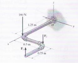
12.  $F_1$ =4 kN and  $F_2$ =2.5 kN,if the resultant force of the three parallel force system acting on the plate is -8.5j kN then the x,z location of the resultant force in meters is :
