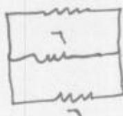
$$R_{\text{eq}} = \frac{1}{\frac{1}{6} + \frac{1}{6}} = \frac{1}{\frac{1}{3}} = 3 \Omega$$
