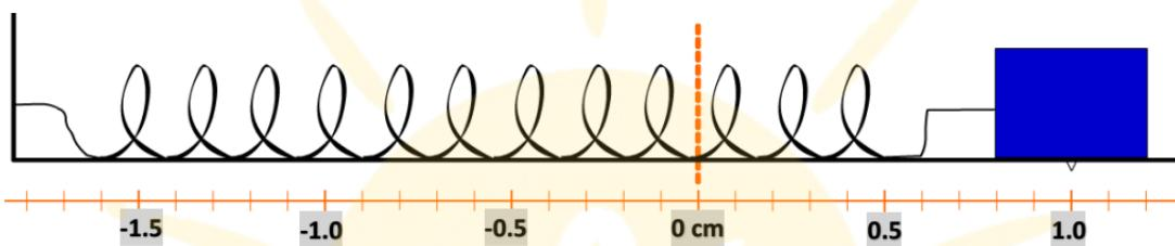
$$a_{max} = \omega^2 A \Rightarrow 0.16 = \omega^2 \times 0.01 \Rightarrow \omega^2 = 16 \Rightarrow \omega = 4 \text{ rad/s}$$
