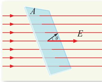
المعطيات:  $E = 100 \text{ N/C}$ ,  $A = 0.05 \times 0.1 \text{ m}^2$ ,  $\theta = 37^\circ$
