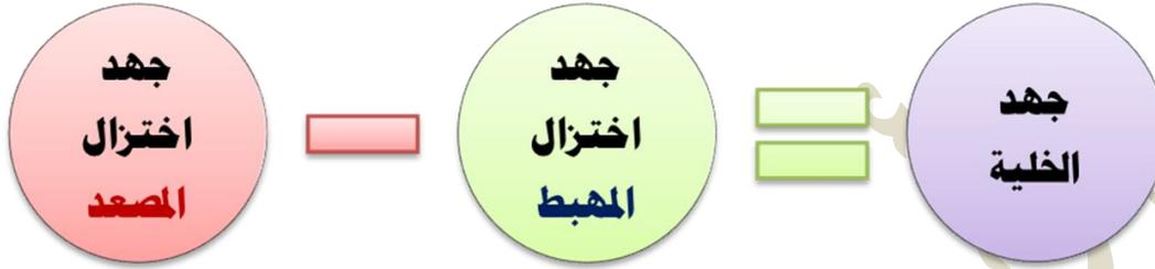
$$E_{\text{cell}} = E_{\text{reduction(cathode)}} - E_{\text{reduction(anode)}}$$
